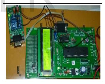
Fig 3 PIC INTERFACING WITH ZIGBEE (BUS STOP)
